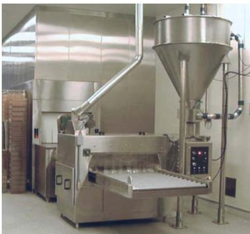
**Automatic Conveyorized Type for use with Tunnel Type Cage Washers**
